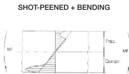
Fig. 21 – Shot-Peened Component Subjected to Bending
